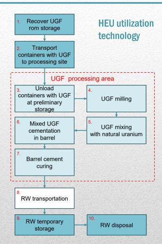
In order to dispose irradiated fuel of the reactor, Kazakhstan specialists have developed a technology of dry mixing, which in the future will solve the issue of irradiated graphite fuel disposition
